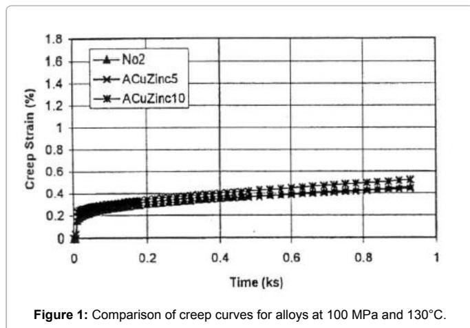
Figure 1: Comparison of creep curves for alloys at 100 MPa and 130°C.
