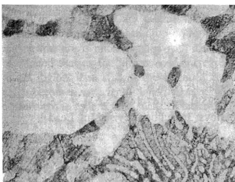
Figure 5: Optical micrograph of ACuZinc5 tested at 100 MPa and 160°C, at high magnification, showing primary ε dendrites and massive η particles with eutectic.
