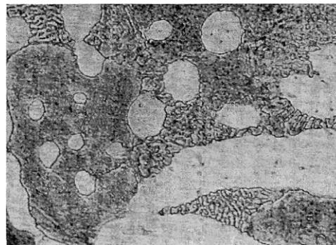
Figure 6: Optical micrograph of ACuZinc10 tested at 100 MPa and 160°C, at high magnification, showing primary ε dendrites and ternary eutectic.
