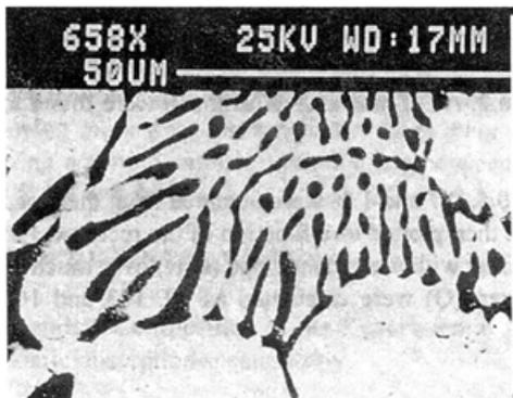
Figure 3: High magnification. SEM micrograph of alloy No.2 tested at 100 MPa and 160°C.
