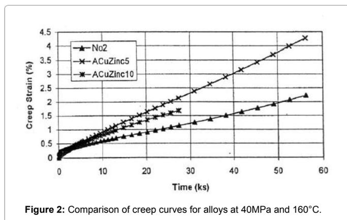
Figure 2: Comparison of creep curves for alloys at 40MPa and 160°C.
