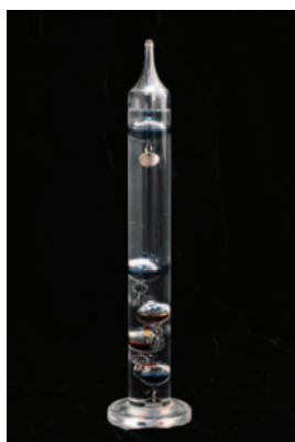
Figure 1: A Galilean thermo scope. A desk-top replica reading in the range of 17°-27°C, with an accuracy of 1°C.
