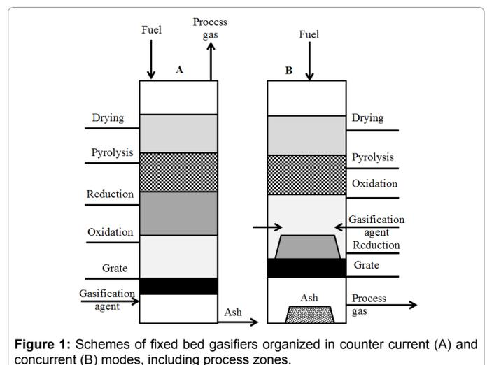
Figure 1: Schemes of fixed bed gasifiers organized in counter current (A) and concurrent (B) modes, including process zones.
