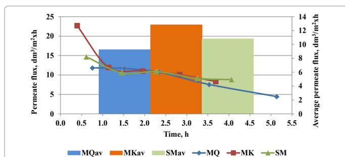
Figure 4: The change and the average capacity of gasification wastewater ultrafiltration.
