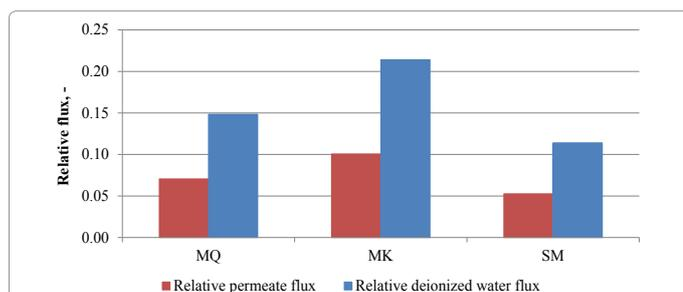
Figure 5: Comparison of relative permeate flux and relative deionized water flux.
