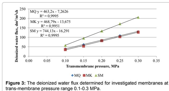
Figure 3: The deionized water flux determined for investigated membranes at trans-membrane pressure range 0.1-0.3 MPa.
