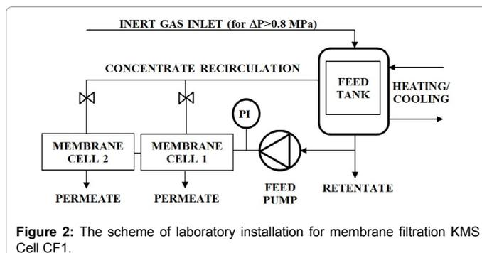
Figure 2: The scheme of laboratory installation for membrane filtration KMS Cell CF1.
