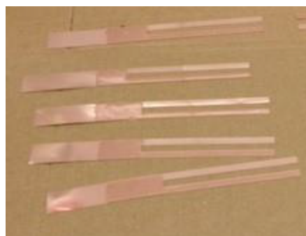
Figure 1: Copper strips having strip constant of 0.3449 with one side of the legs varnished.
