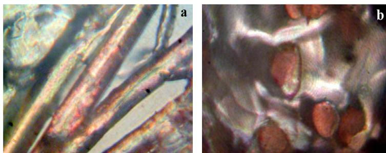
Figure 7: Images (100X) of polyester substrate treated with nano-cellulose and stained with congo red direct dye (a) longitudinal and (b) cross sectional view.
