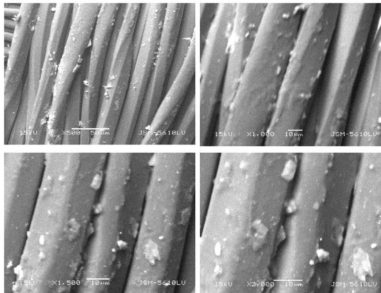
Figure 8: Polyester fiber surface morphology after treatment with the nano-cellulose treatment.
