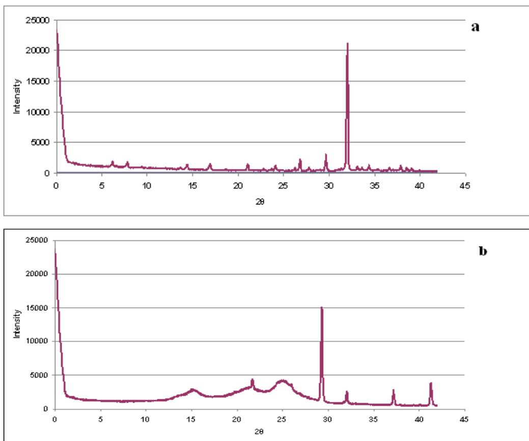
Figure 10: X-ray diffraction pattern of a) pure polyester and b) polyester treated with nano cellulose.
