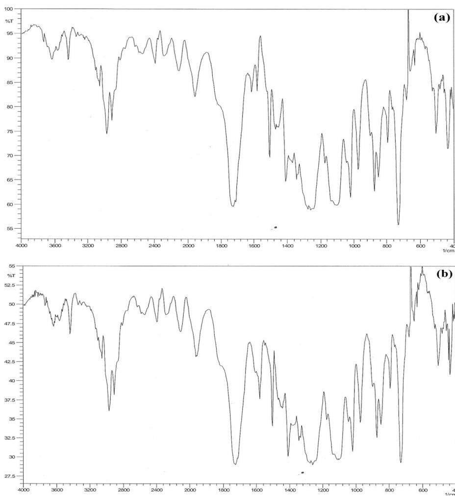
Figure 9: FTIR spectra of (a) pure polyester fabric and (b) polyester fabric treated with nano-cellulose.
