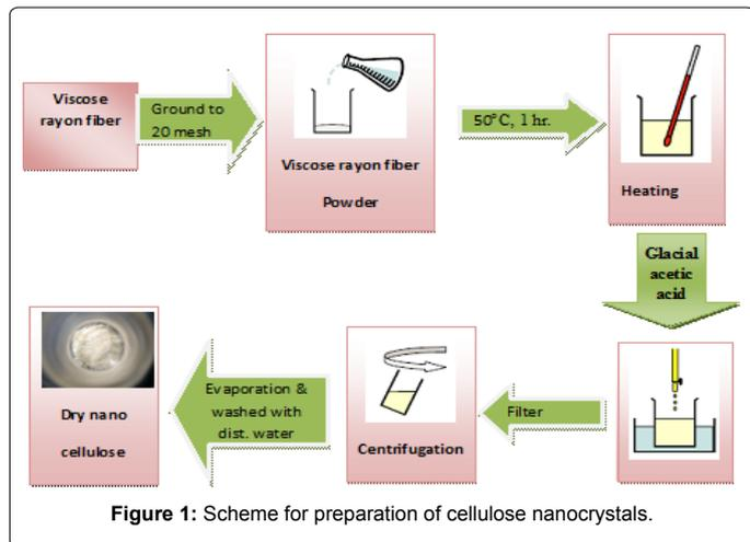
Figure 1: Scheme for preparation of cellulose nanocrystals.
