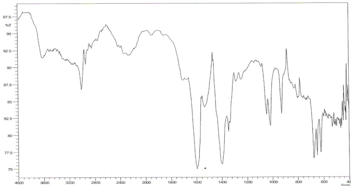
Figure 5: IR Characterization absorption peak of prepared nano cellulose powder.
