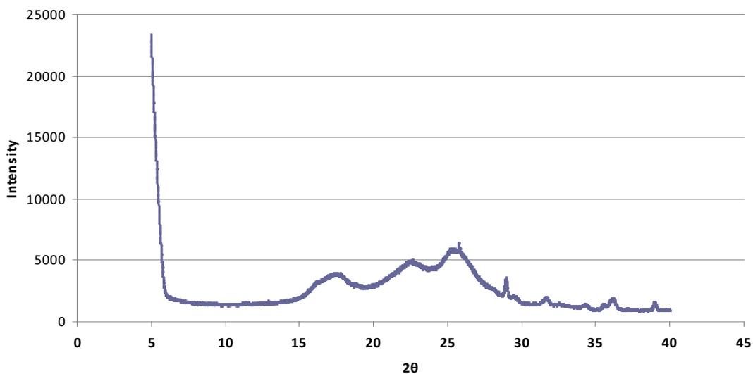
Figure 6: X-ray diffraction pattern of nano cellulose.
