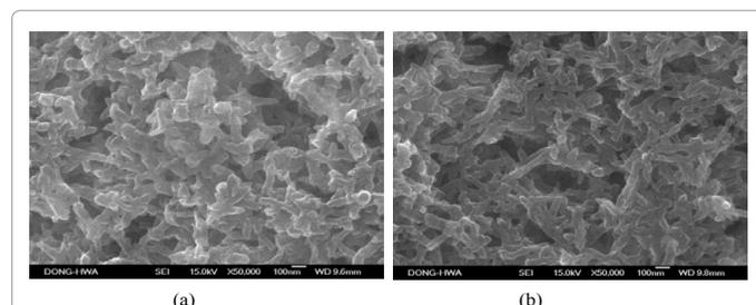
**Figure 1:** FE-SEM images of the (a)  $PANIM_0$  (b)  $PANIM_{1.5}$  samples at X50000 magnification.
