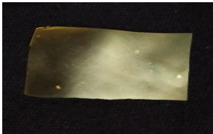
Figure 6. Edible film prepared by 2.5% glycerol concentration and ratio of chitosan of 1.2: 0.8.
