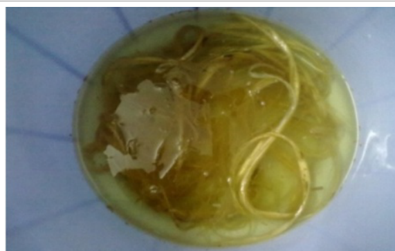
Figure 3: Treatment of Fiber in 2% NaOH solution.
