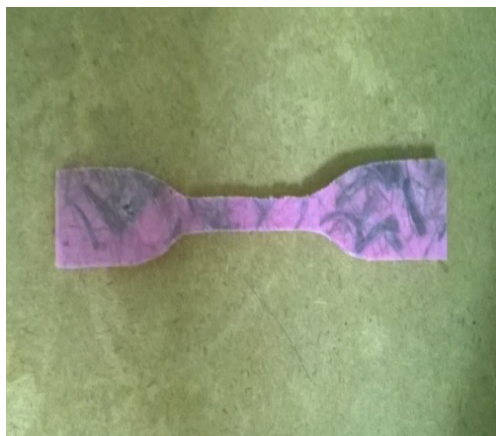
Figure 9: Tensile test specimen ASTM D-638.
