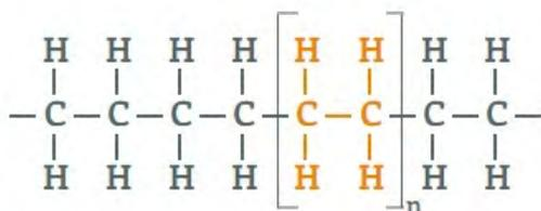
Figure 4. Molecular structure of PE
