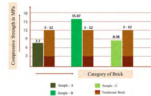
**Figure 13.** Comparison of compressive strength of developed and traditional brick
