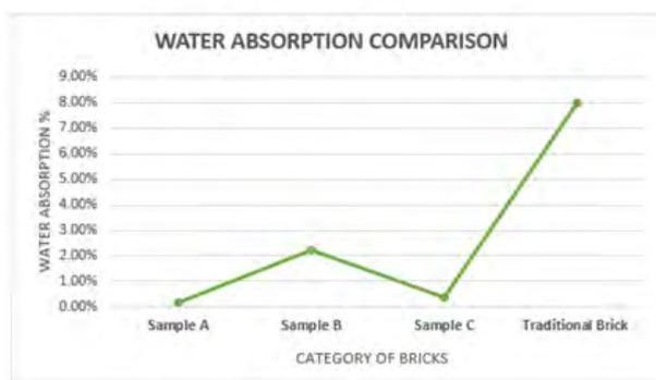
**Figure 14.** Comparison of water absorption % of developed and traditional brick
