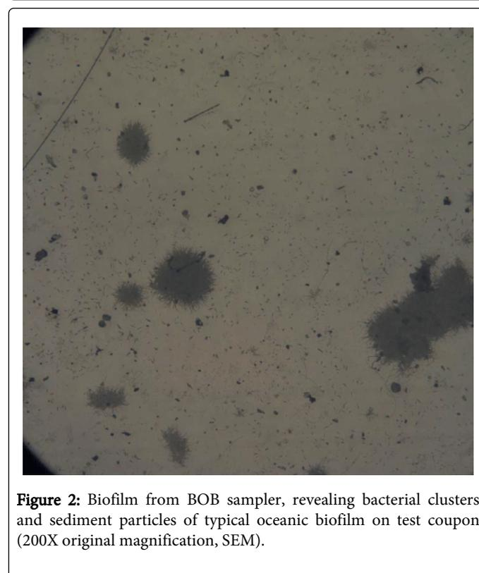
**Figure 2:** Biofilm from BOB sampler, revealing bacterial clusters and sediment particles of typical oceanic biofilm on test coupon (200X original magnification, SEM).
