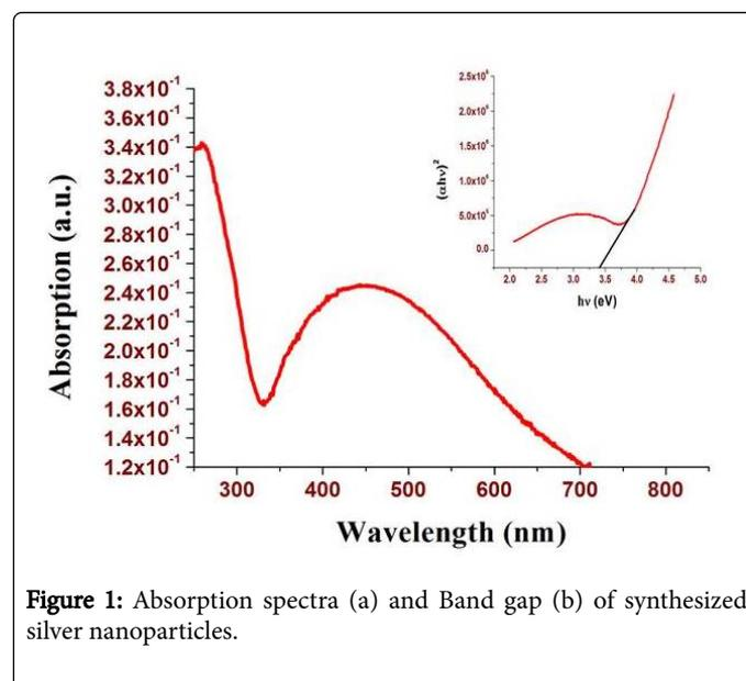
Figure 1: Absorption spectra (a) and Band gap (b) of synthesized silver nanoparticles.
