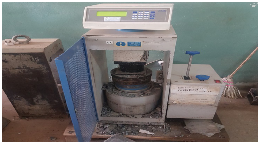
Figure 7. Specimens for compressive strength.
