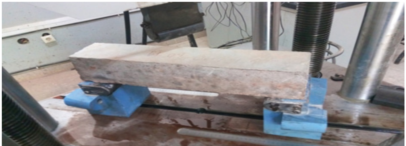
Figure 9. Specimens during testing for flexure.
