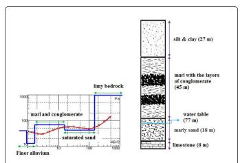
Figure 7: Compare of VES (sounding 170) with the geological sections.
