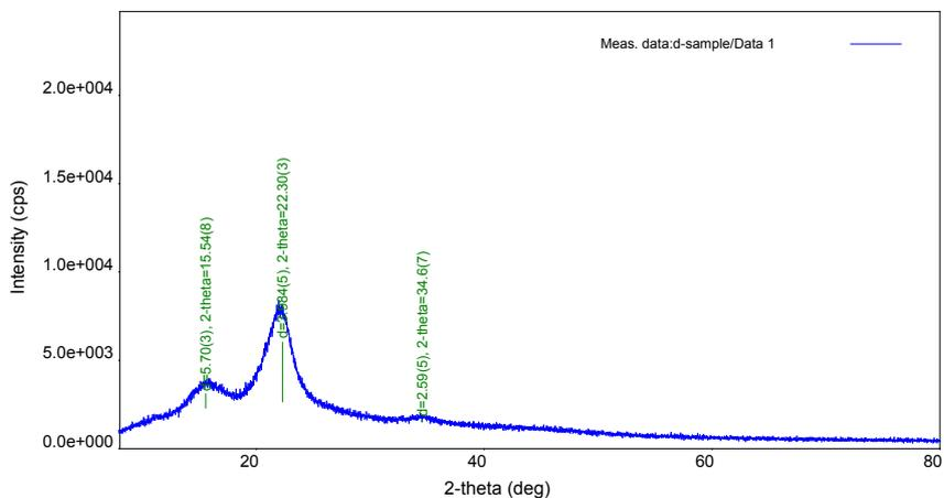
Figure 2d: XRD of Chemical Assisted Natural retted bamboo fibres after treatment D [20 g/L NaOH in the presence of 5 g/L Sodium tri phosphate solution (Na<sub>3</sub>P<sub>3</sub>O<sub>10</sub>)].
