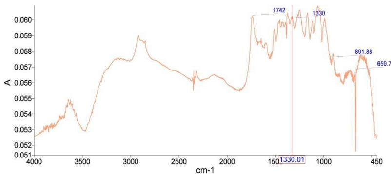
Figure 1c: FTIR of Chemical Assisted Natural retted bamboo fibres after treatment C [with 0.7% (on the weight of fibres) NaClO<sub>2</sub> solution (Sodium chlorite solution)].
