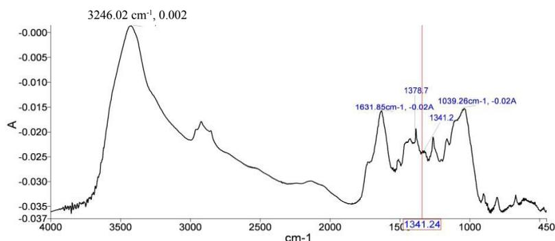
Figure 1: (CAN): FTIR of Chemical Assisted Natural retted bamboo fibres.
