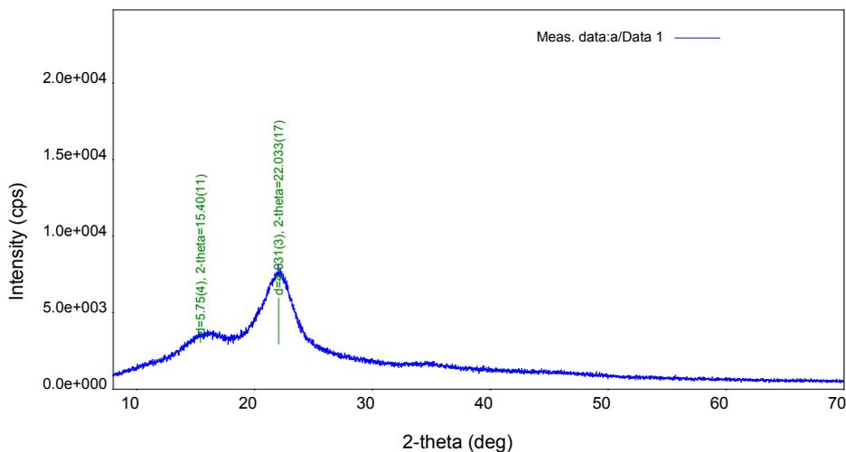
Figure 2b: XRD of Chemical Assisted Natural retted bamboo fibres after treatment B (solution 0.1N NaOH).
