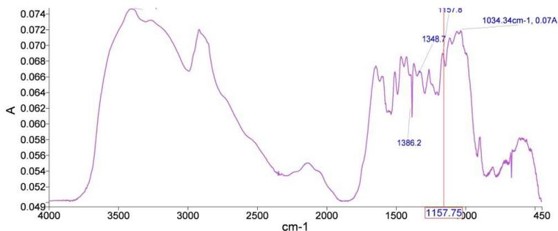
Figure 1e: FTIR of Chemical Assisted Natural retted bamboo fibres after treatment E (150 g/L NaOH solution).
