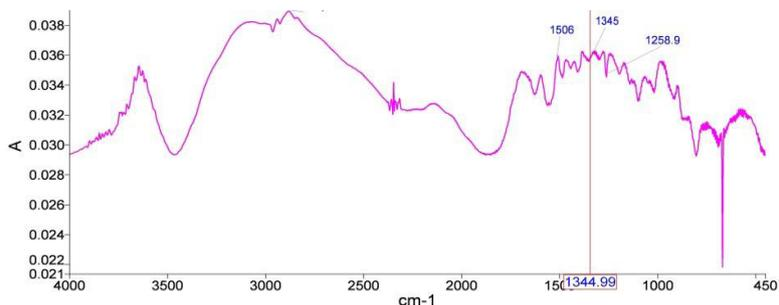
Figure 1b: FTIR of Chemical Assisted Natural retted bamboo fibres after treatment B (solution 0.1N NaOH).
