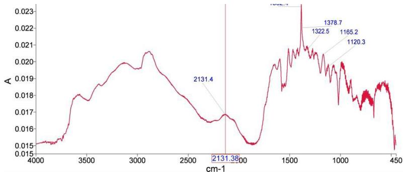
Figure 1d: FTIR of Chemical Assisted Natural retted bamboo fibres after treatment D [20 g/L NaOH in the presence of 5 g/L Sodium tri phosphate solution (Na<sub>5</sub>P<sub>3</sub>O<sub>10</sub>)].
