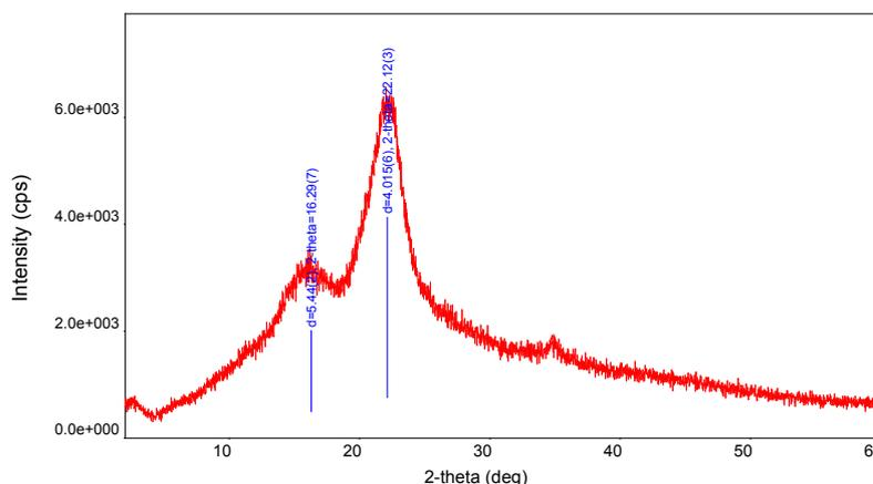
Figure 2: CAN. XRD of Chemical Assisted Natural retted bamboo fibres (CAN) without treatment.
