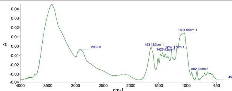
Figure 1a: FTIR of Chemical Assisted Natural retted bamboo fibres after treatment A [mixture of 17.5% (on the weight of fibres) NaOH and 17.5% (on the weight of fibres) KOH solution].
