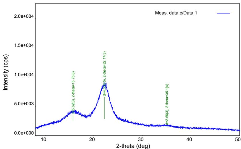
Figure 2c: XRD of Chemical Assisted Natural retted bamboo fibres after treatment C [with 0.7% (on the weight of fibres) NaClO<sub>2</sub> solution (Sodium chlorite solution)].
