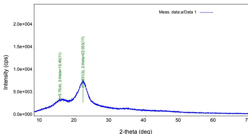
Figure 2a: XRD of Chemical Assisted Natural retted bamboo fibres after treatment A [mixture of 17.5% (on the weight of fibres) NaOH and 17.5% (on the weight of fibres) KOH].
