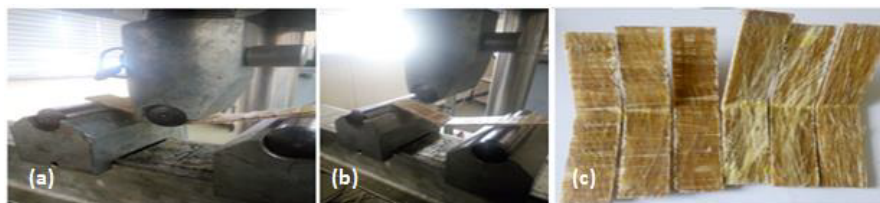
Figure 3: (a) Fixture of the three point (flexural) test before loaded (b) fixture of flexural test after loaded (c) fracture mode of specimen.
