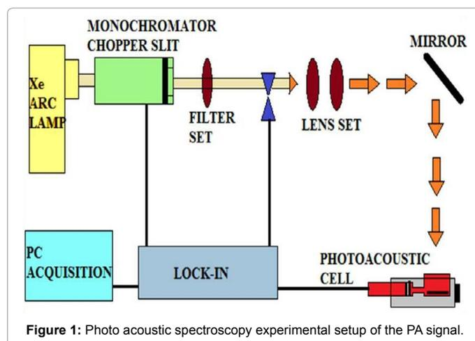
Figure 1: Photo acoustic spectroscopy experimental setup of the PA signal.
