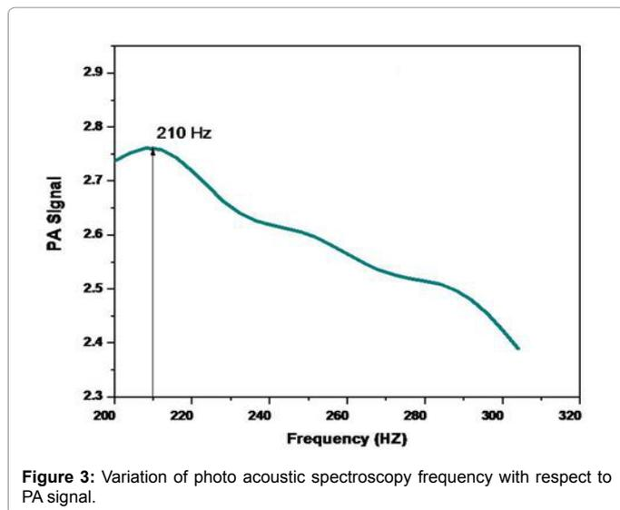
Figure 3: Variation of photo acoustic spectroscopy frequency with respect to PA signal.
