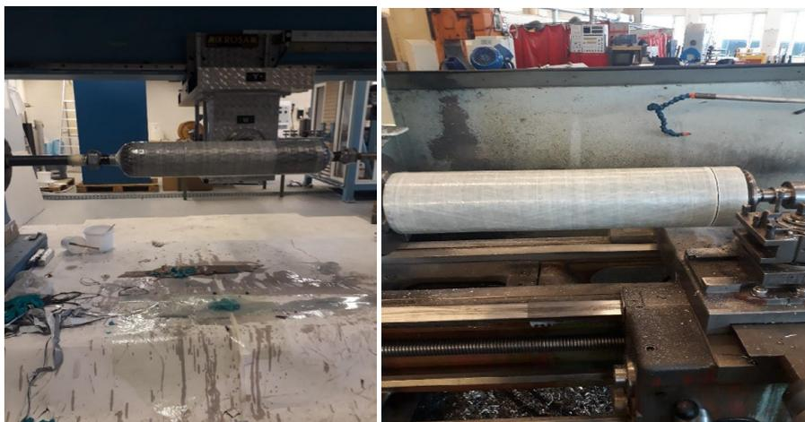
Figure 9: Winding of Glass Fiber at 90° left side and Cutting of Test Sample for fatigue testing after hardening at the right side.
