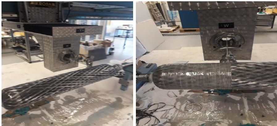
Figure 8: Winding of Glass Fiber at 15° at left and 90° right side.
