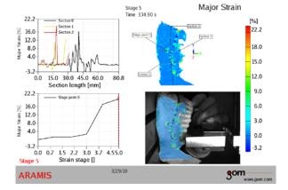
Figure 5: Major strain field within the fifth of the restored mandible loading
