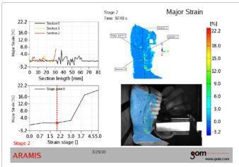
Figure 2: Major strain field within the second of the restored mandible loading
