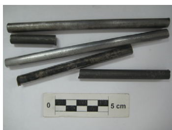
Figure 1: Segments of steel wire 30MnB5 of starting.
