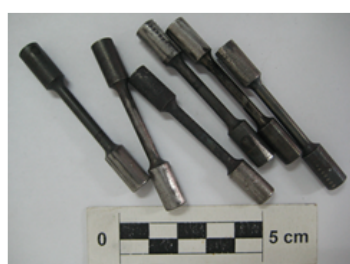
Figure 3: Samples machined for tensile testing, heat treated.
