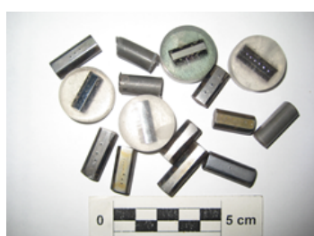
Figure 2: Specimens taken from the starting wire, heat treated, examined and tested by metallographic tests of hardness and microhardness.
