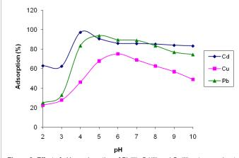
Figure 3: Effect of pH on adsorption of Pb(II), Cd(II) and Cu(II) onto raw wheat straw. (metal concentration: 50 mg/L; contact time: 15 min; agitation speed: 100 rpm; temperature: 303 K; dose: 0.4g/50mL for Pb(II), 0.6g/50mL for Cd(II) and Cu(II)).
