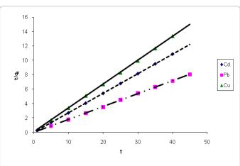
**Figure 6:** Pseudo second-order kinetic plot for the adsorption of Pb(II), Cd(II) and Cu(II) on raw wheat straw. (metal concentration: 50 mg/L; dose 0.4g/50mL for Pb(II), 0.6 g/50mL for Cd(II) and Cu(II); contact time: 20 min for Pb(II), 10 min for Cd(II), 25 min for Cu(II); temperature: 303 K).
