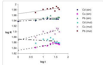
**Figure 7:** Intra-particle diffusion model for the adsorption of Pb(II), Cd(II) and Cu(II) on raw wheat straw in single and multi-component system. (metal concentration: 50 mg/L; dose 0.4g/50mL for Pb(II), 0.6 g/50mL for Cd(II) and Cu(II); contact time: 20 min for Pb(II), 10 min for Cd(II), 25 min for Cu(II); temperature: 303 K).
