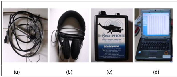
Figure 5: Set voice recorders, (a) Hydrophone, (b) Headphone, (c) the power supply/battery, and (d) laptop for data logging and data processing [17].
