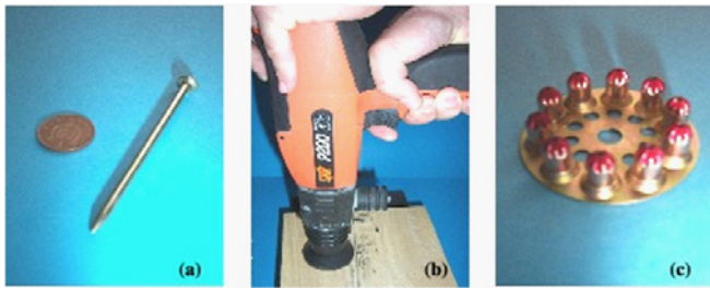
Figure 2: (a) An example of the high strength steel nails used in the flitch joint tests, (b) the nailing gun and (c) the nails are fired through the composite by means of a forceful explosion delivered by these charges.
