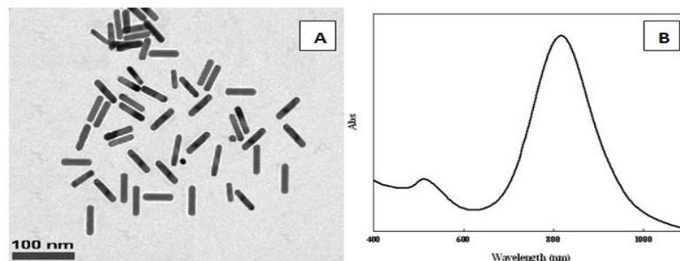
Figure 2: Electron microscopic shape of gold nanorods TEM images (A), and absorption spectra of aqueous of 10nm AuNRs solution (B).
