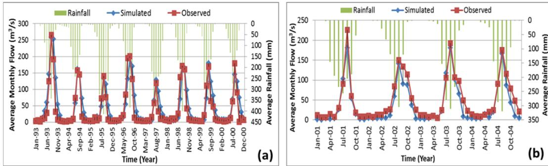
Figure 4: Calibration (a) and validation (b) results of average monthly observed and simulated stream flows at the outlet of Hombole gauged station.
