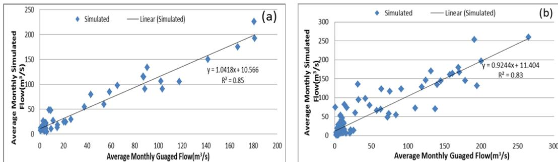
Figure 5: Scatter plot of monthly gauged versus simulated flow at Hombole gauged station for (a) calibration and (b) validation periods.
