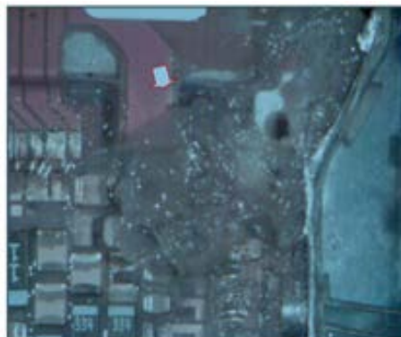
Figure 5: Opened can with body fluids inside of titanium case and noted on the hybrid.
