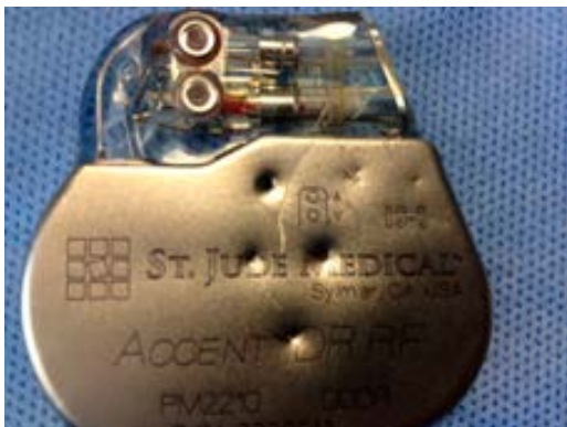
Figure 2: Front view of can post explant. Arrows indicate penetration of titanium Pulse generator case.
