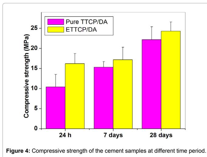
**Figure 4:** Compressive strength of the cement samples at different time period.
