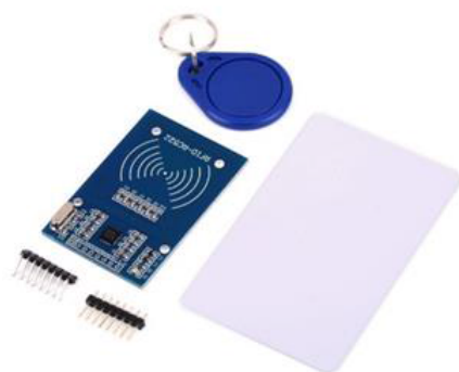
Figure 5: RFID RC522 with tags.
