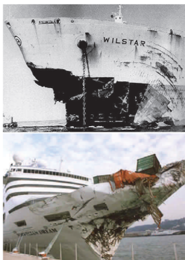
Figure 2: (Top): The Wilstar after being hit by a rogue wave in the Agulhas current outside South Africa in 1974. (Bottom): More recently, the Norwegian Dream suffered heavy damage while returning to New York from a cruise in 2005.
