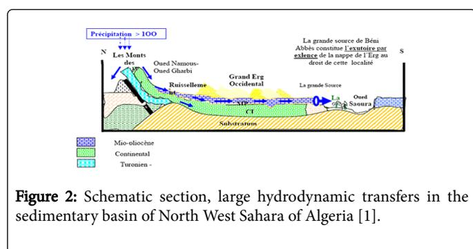
Figure 2: Schematic section, large hydrodynamic transfers in the sedimentary basin of North West Sahara of Algeria [1].
