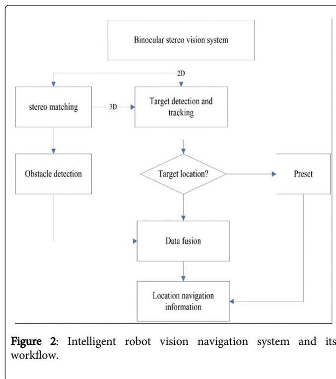
**Figure 2:** Intelligent robot vision navigation system and its workflow.
