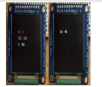
Figure 3: Demonstration of OLED display dynamically displaying MCM data.
