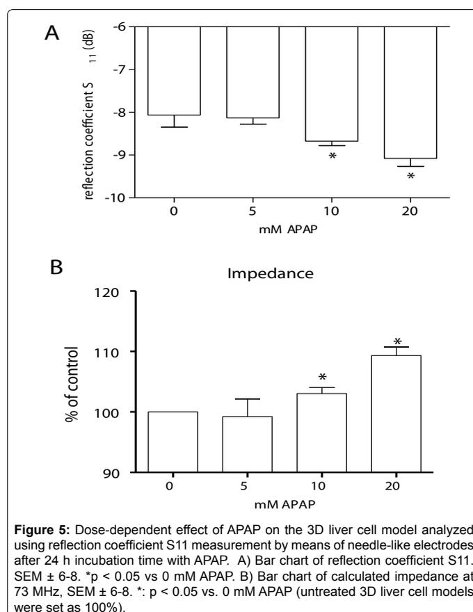
**Figure 5:** Dose-dependent effect of APAP on the 3D liver cell model analyzed using reflection coefficient S11 measurement by means of needle-like electrodes after 24 h incubation time with APAP. A) Bar chart of reflection coefficient S11. SEM  $\pm$  6-8. \* $p < 0.05$  vs 0 mM APAP. B) Bar chart of calculated impedance at 73 MHz, SEM  $\pm$  6-8. \*:  $p < 0.05$  vs. 0 mM APAP (untreated 3D liver cell models were set as 100%).
