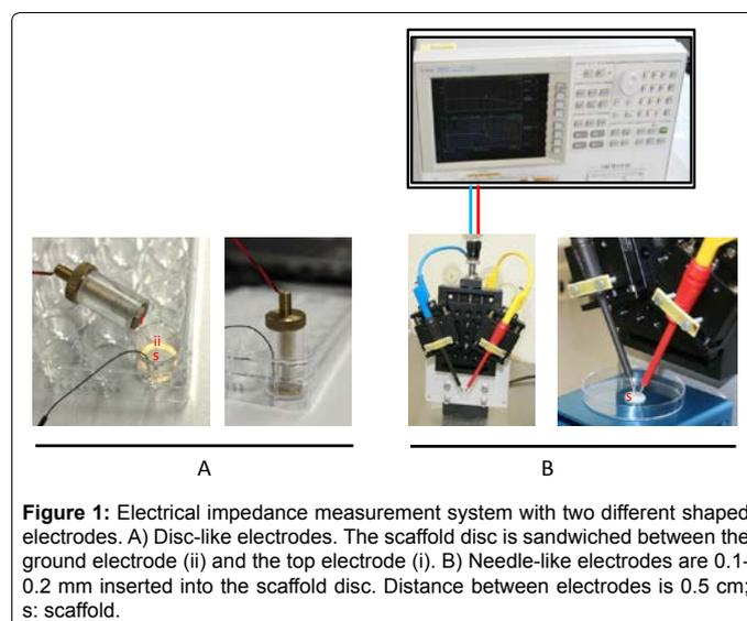
**Figure 1:** Electrical impedance measurement system with two different shaped electrodes. A) Disc-like electrodes. The scaffold disc is sandwiched between the ground electrode (ii) and the top electrode (i). B) Needle-like electrodes are 0.1-0.2 mm inserted into the scaffold disc. Distance between electrodes is 0.5 cm; s: scaffold.
