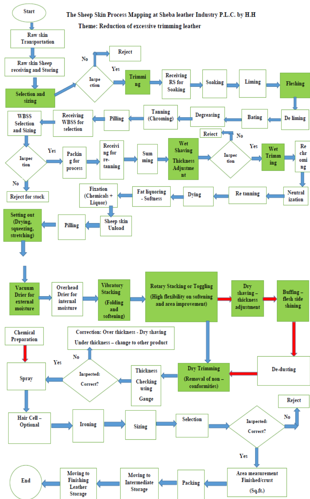
Figure 3: Process flow of leather making in Sheba.
