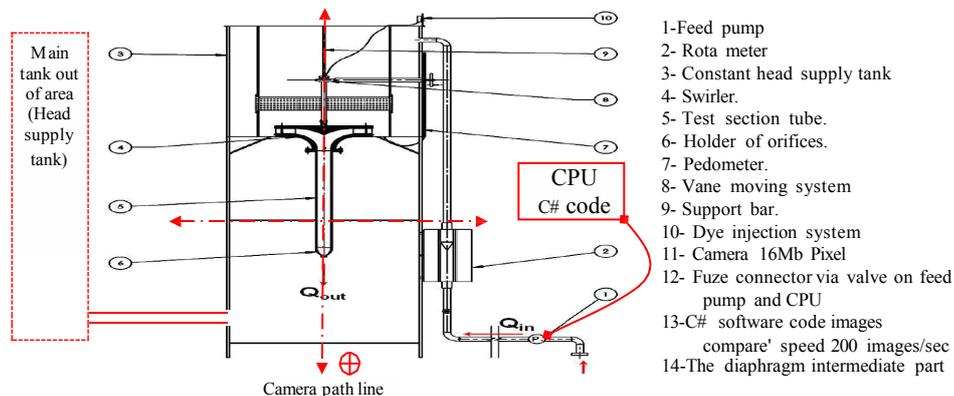
Figure 5: Prototype device used in controlling system experimentally.
