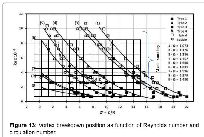
Figure 13: Vortex breakdown position as function of Reynolds number and circulation number.
