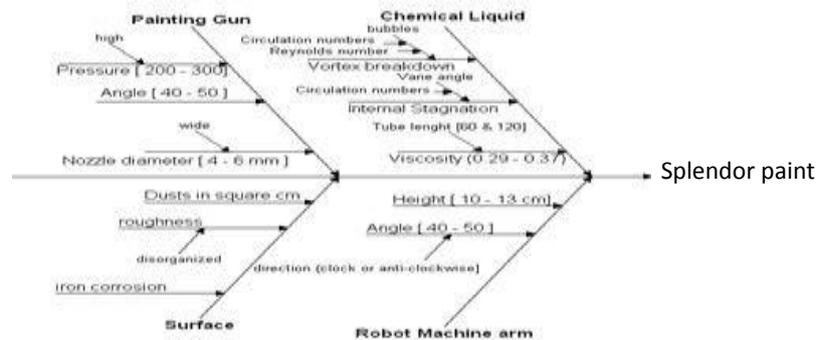
Figure 3: Cause and effect of painting Ibeam bathtubs model.
