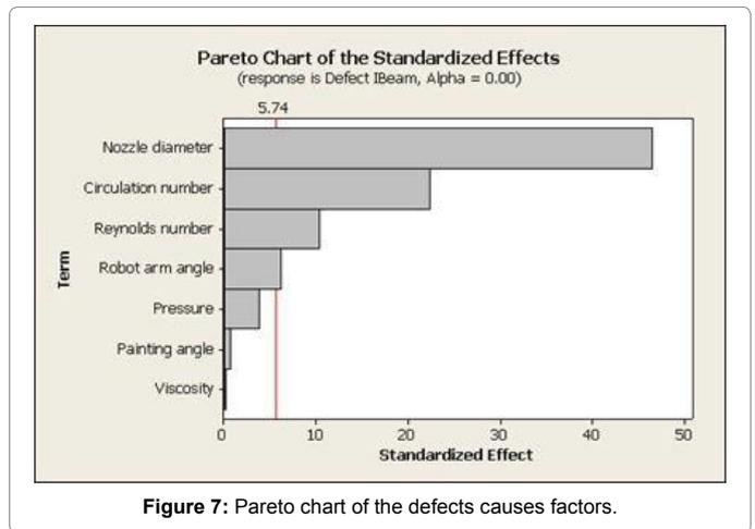
Figure 7: Pareto chart of the defects causes factors.
