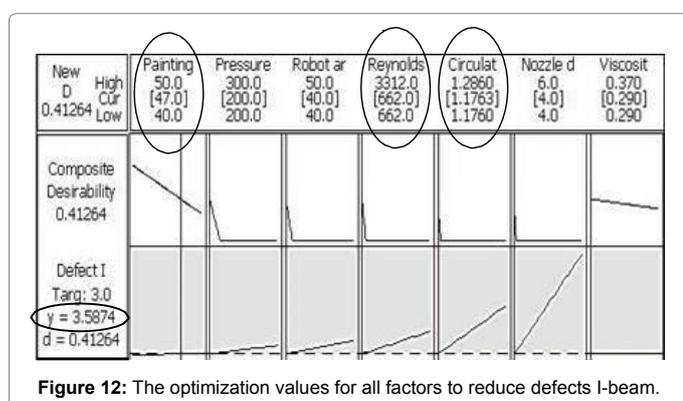
Figure 12: The optimization values for all factors to reduce defects I-beam.
