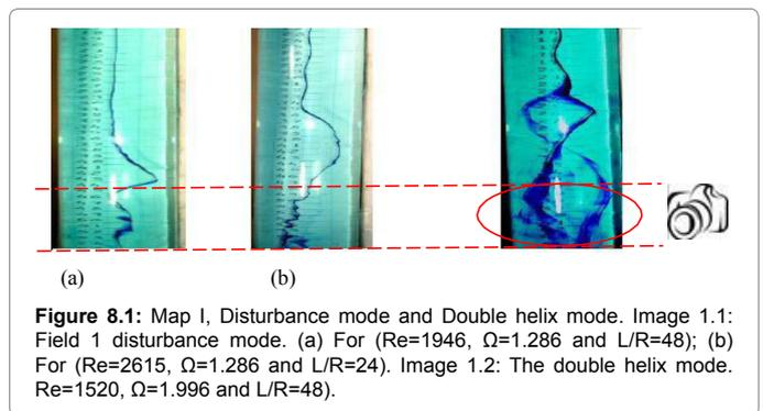
Figure 8.1: Map I, Disturbance mode and Double helix mode. Image 1.1: Field 1 disturbance mode. (a) For (Re=1946,  $\Omega=1.286$  and  $L/R=48$ ); (b) For (Re=2615,  $\Omega=1.286$  and  $L/R=24$ ). Image 1.2: The double helix mode. Re=1520,  $\Omega=1.996$  and  $L/R=48$ .
