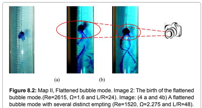
Figure 8.2: Map II, Flattened bubble mode. Image 2: The birth of the flattened bubble mode.(Re=2615,  $\Omega=1.6$  and  $L/R=24$ ). Image: (4 a and 4b) A flattened bubble mode with several distinct emptying (Re=1520,  $\Omega=2.275$  and  $L/R=48$ ).
