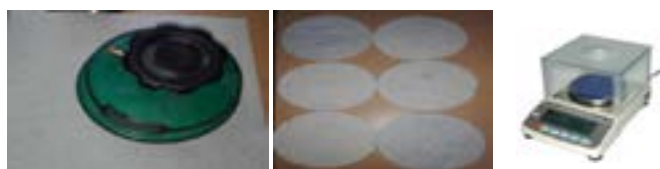
Figure 9. Nonwoven fabric weight testing.
