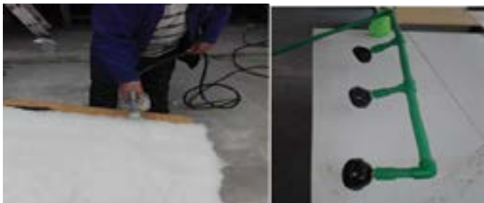
Figure 6. Adhesive bonding of recycled selvage waste nonwovens.
