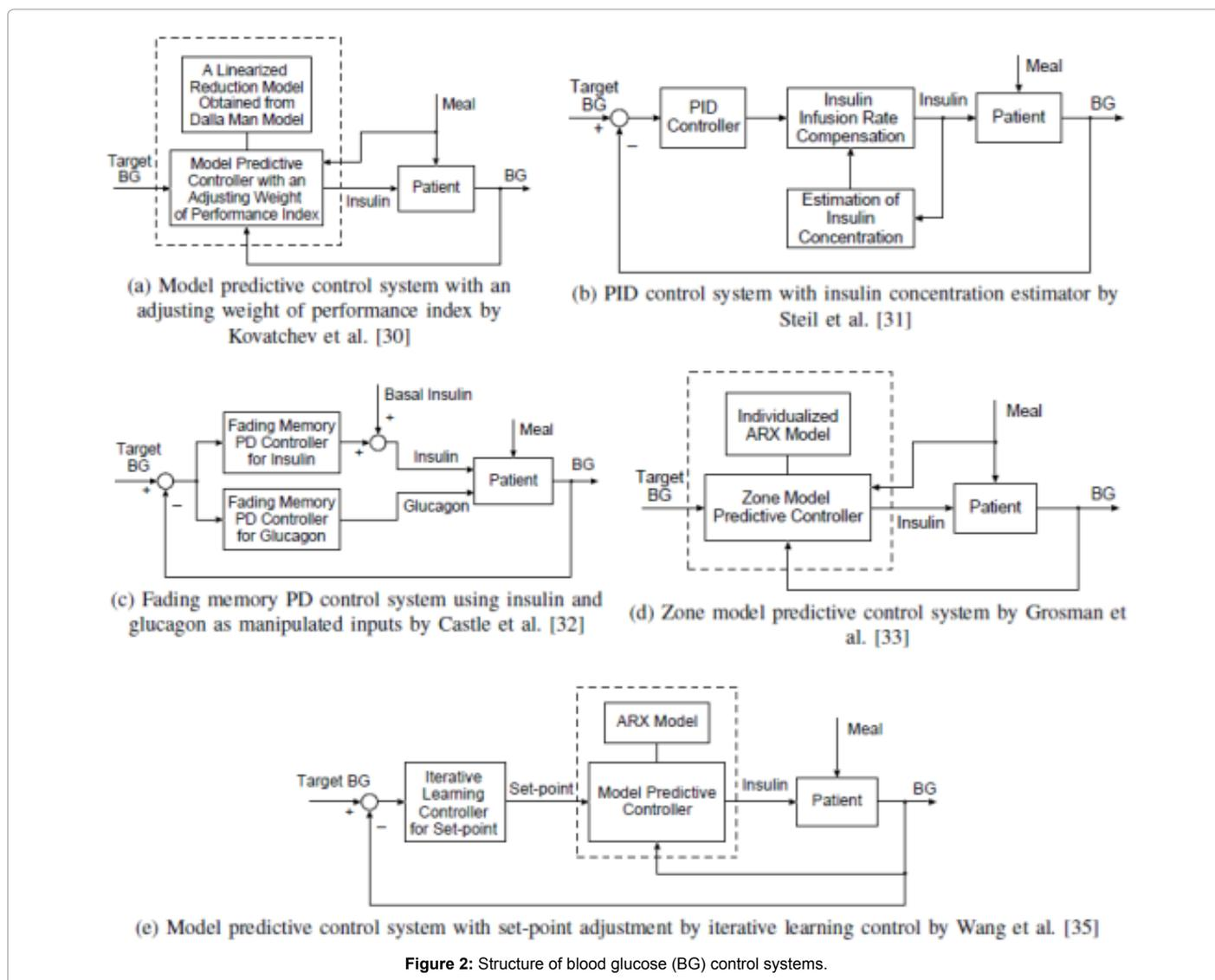
Figure 2: Structure of blood glucose (BG) control systems.
