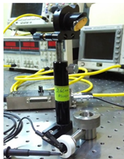
Figure 3. Close view of the gold coated beam folding mirror and PA cell coupled to microphone detector.
