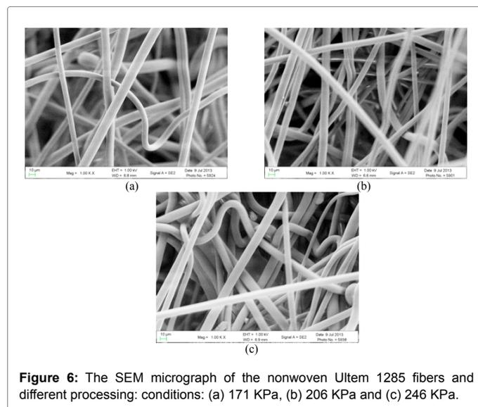
Figure 6: The SEM micrograph of the nonwoven Ultem 1285 fibers and different processing: conditions: (a) 171 KPa, (b) 206 KPa and (c) 246 KPa.
