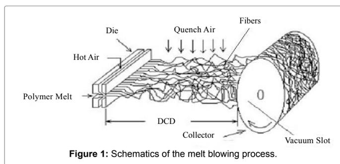
Figure 1: Schematics of the melt blowing process.
