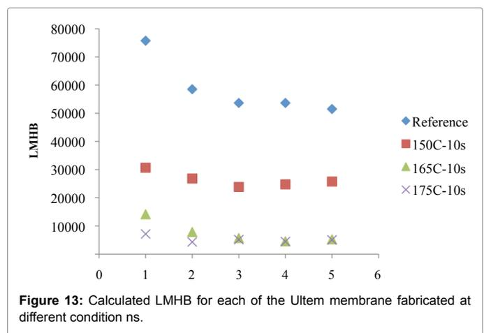
Figure 13: Calculated LMHB for each of the Ultem membrane fabricated at different condition ns.
