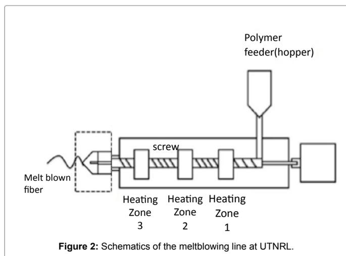
Figure 2: Schematics of the meltblowing line at UTNRL.
