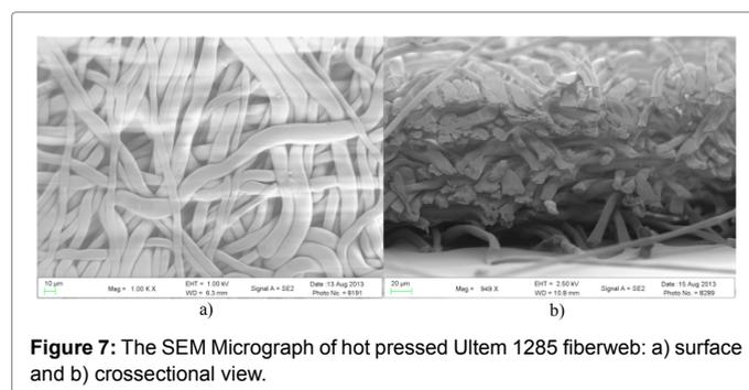
Figure 7: The SEM Micrograph of hot pressed Ultem 1285 fiberweb: a) surface and b) crosssectional view.
