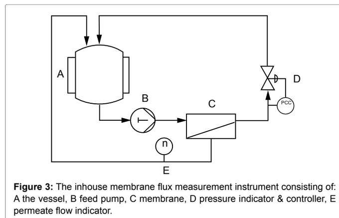
Figure 3: The inhouse membrane flux measurement instrument consisting of: A the vessel, B feed pump, C membrane, D pressure indicator & controller, E permeate flow indicator.
