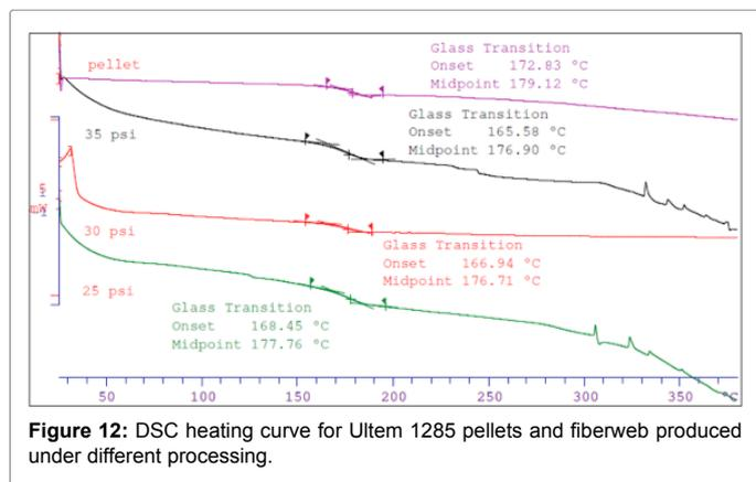
Figure 12: DSC heating curve for Ultem 1285 pellets and fiberweb produced under different processing.
