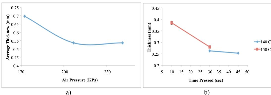
Figure 9: The relationship between the thickness of the resulting Ultem 1285 meltblown webs: a) meltblowing pressure, and b) the calendering temperature/time.
