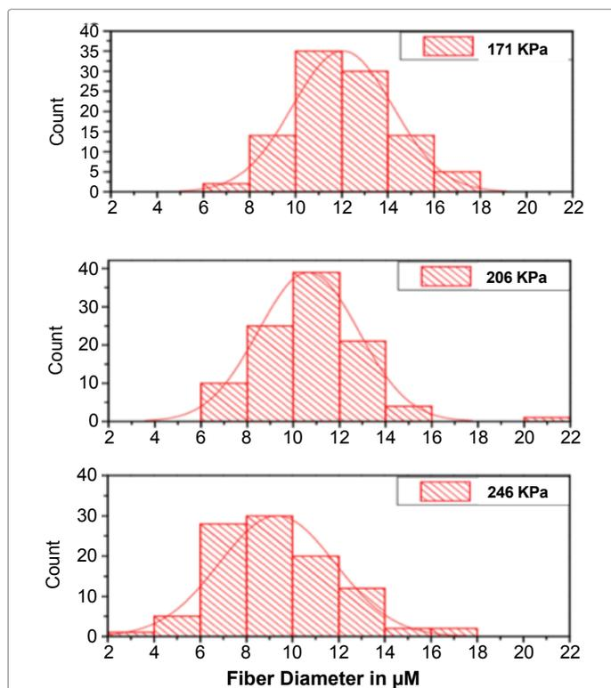
Figure 5: Fiber diameter and diameter distribution.
