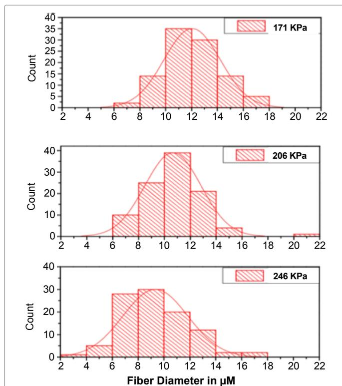
Figure 5: Fiber diameter and diameter distribution.
