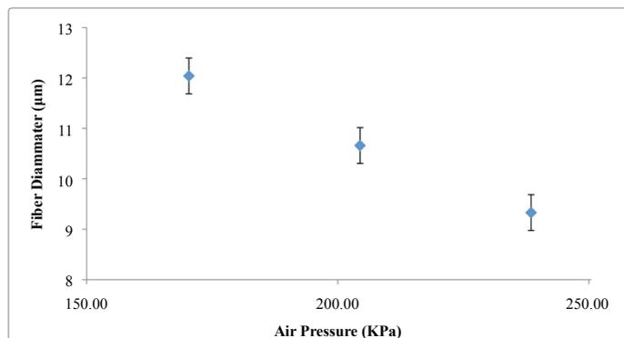
Figure 4: The relationship between the air pressure and the fiber diameter.
