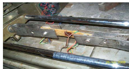
Figure 2: Test specimen mounted on Hounsfield Tensometer.
