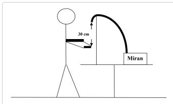
Figure 1: Experimental setup for studying the ambient levels of ethanol associated with the use of HAS.
