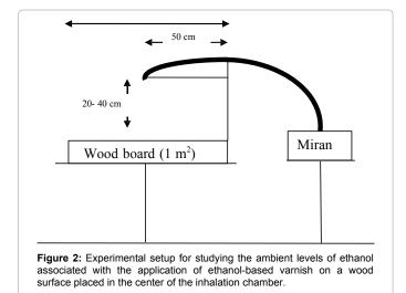
is described in Figure 2. Ethanol in air was measured 20 cm and 40 cm above the center of the board with the infrared spectrophotometer described above. The distance between the sampling point (worker's breathing zone) and the varnished board was chosen arbitrarily. The concentration in the inhalation chamber was also recorded and the measurements were done for an entire 60-minute period.
