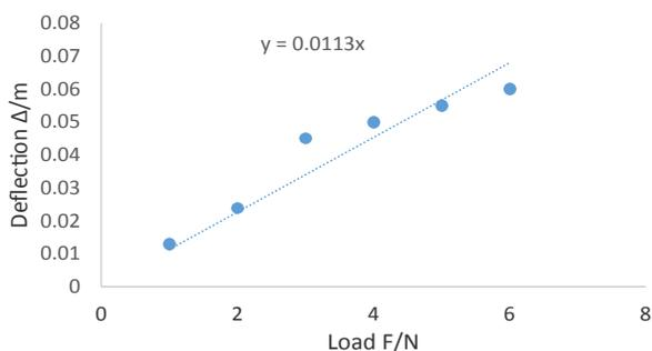
Figure 9: Variation of deflection and load applied for 0.5 m of optic fibre using method 1.
