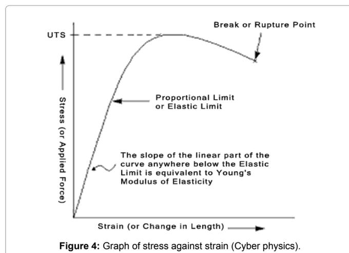
Figure 4: Graph of stress against strain (Cyber physics).
