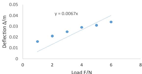
Figure 8: Variation of deflection and load applied for 0.3 m of optic fibre using method 1.
