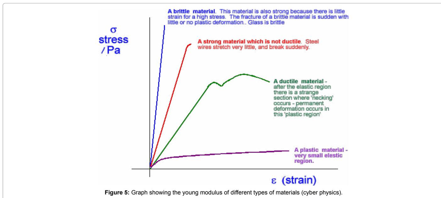
strains e.g. Steel as shown by figure but gradually change as it reaches the various stages. The steepness of the slope determines the strength of the materials. By determining the Young modulus of a material it will help in the material's applicability as this determines how much load it can withstand without failure.
