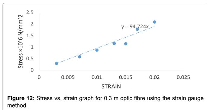
Figure 12: Stress vs. strain graph for 0.3 m optic fibre using the strain gauge method.
