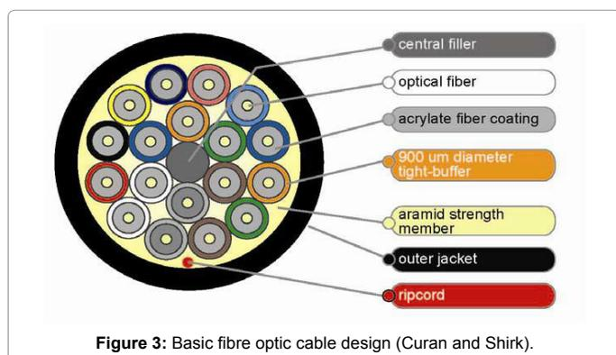
Figure 3: Basic fibre optic cable design (Curan and Shirk).
