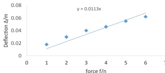
Figure 10: Variation of deflection and load applied for 1.0 m of optic fibre.
