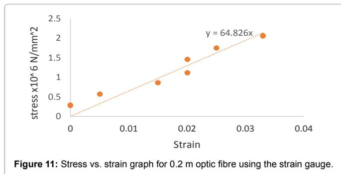
Figure 11: Stress vs. strain graph for 0.2 m optic fibre using the strain gauge.
