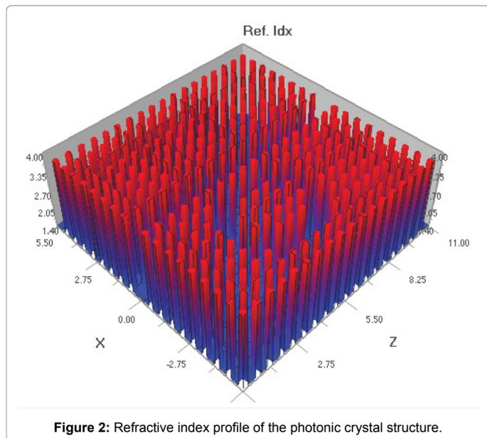
Figure 2: Refractive index profile of the photonic crystal structure.
