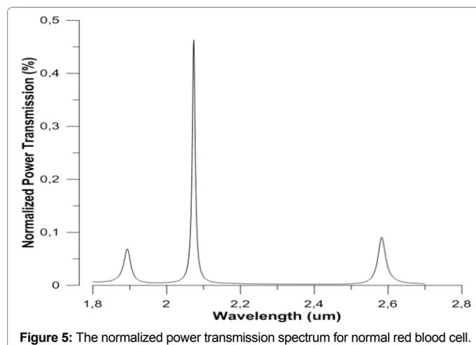
Figure 5: The normalized power transmission spectrum for normal red blood cell.
