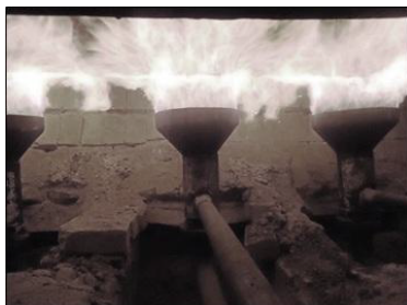
Figure 7: Producer gas flaring burners below rotary kiln.
