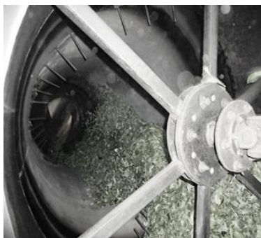
Figure 2: Panning process in rotary drum.
