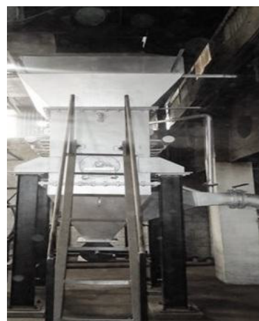
Figure 5: Downdraft gasifier installed for green tea drying.
