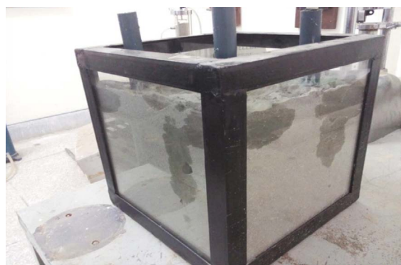
Figure 2: Permeation of cement grouting.
