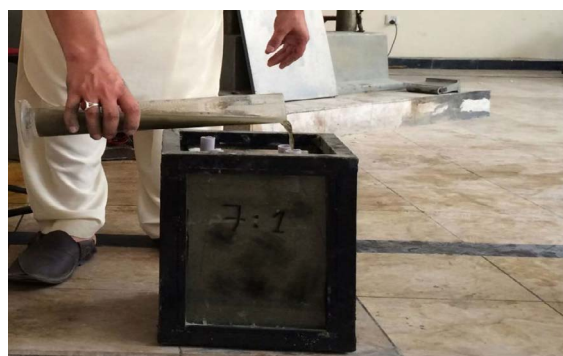
Figure 1: Grout pouring in PVC pipes.
