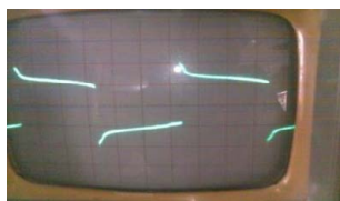
Figure 3: Branded inverter on no load.
