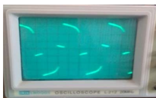
Figure 4: Branded inverter on resistive load.
