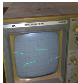
Figure 6: Branded inverter on inductive load.
