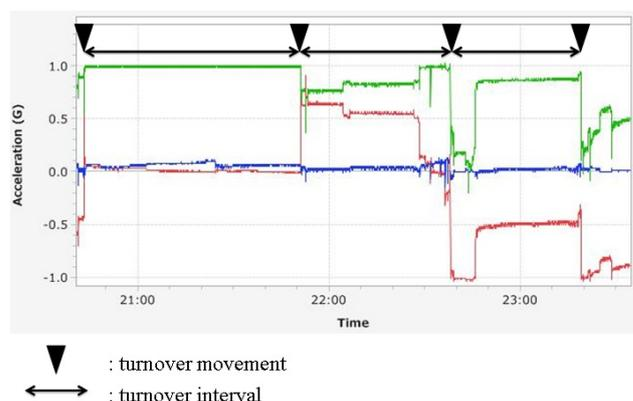
**Figure 3:** Measurement of turnover movements and turnover interval.
