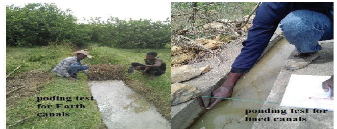
Figure 7. Estimation of seepage losses from irrigation canals using ponding test method.
