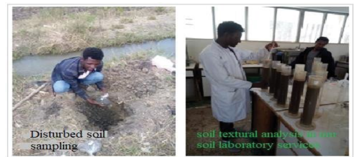
Figure 3. Soil sampling at the canal bank and soil textural analysis at mekelle university soil laboratory service.
