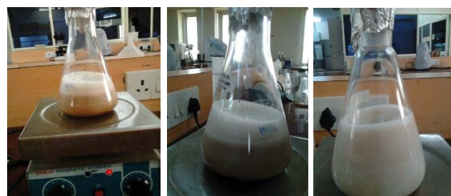
Figure 8: Foam formation using magnetic stirrer after the fermentation in order to enhance bio surfactant production.
