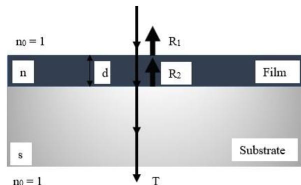
**Figure 1.** Model of a thin film on a transparent substrate
