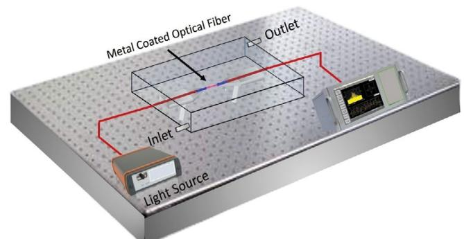
Figure 1. Schematic diagram of optical fiber SPR sensor.
