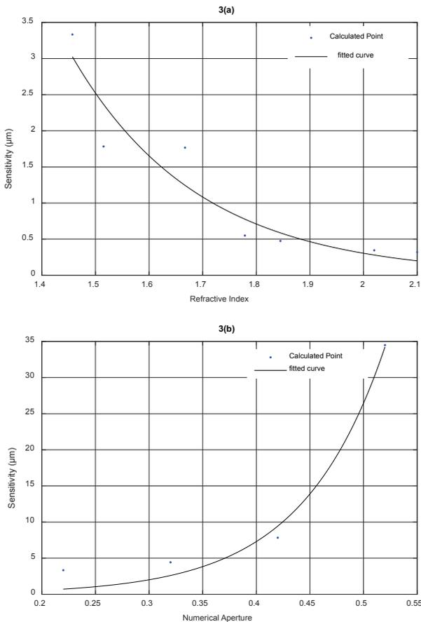
Figure 3. Sensitivity at different core refractive index (a) and numerical aperture (b).
