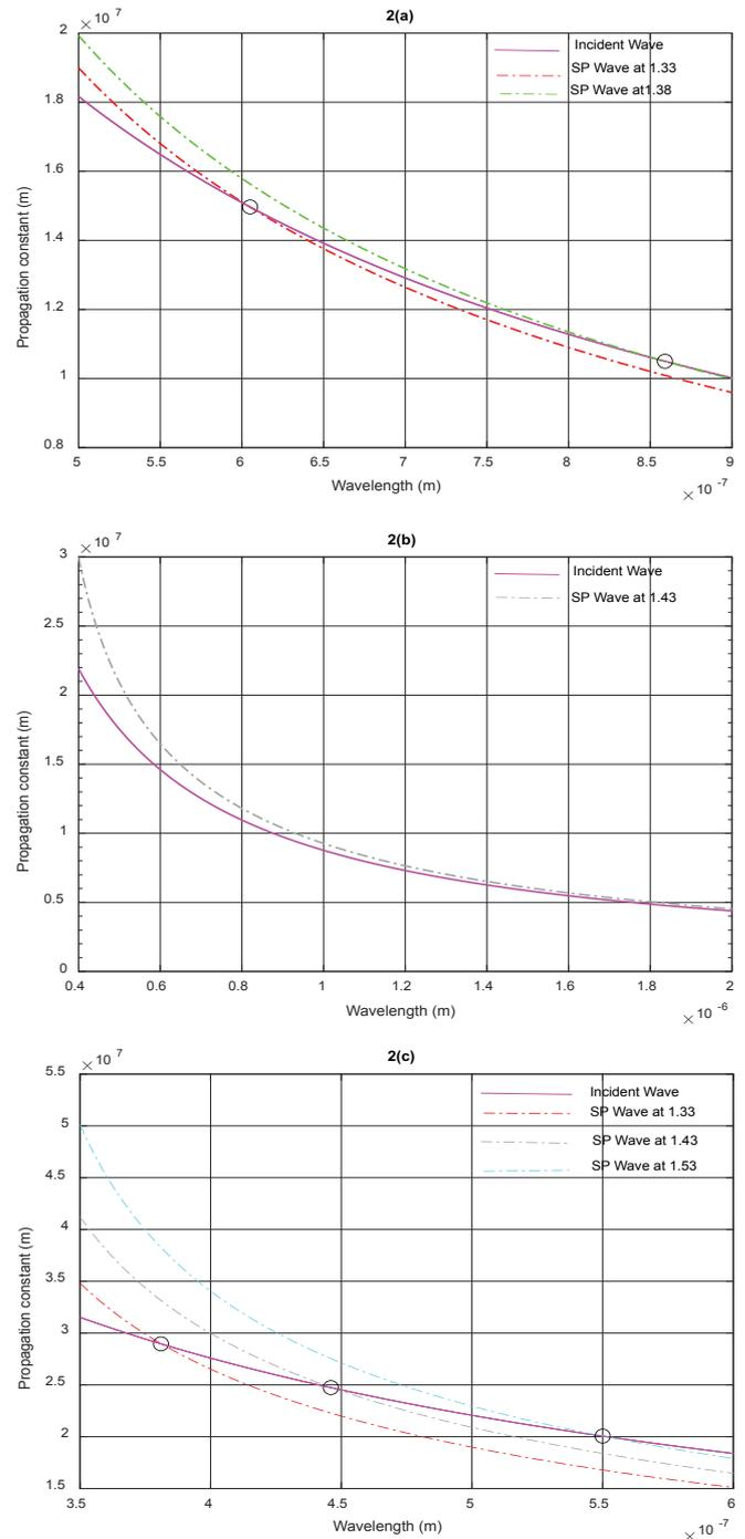
Figure 2. Propagation constant at different wavelength (a-c).
