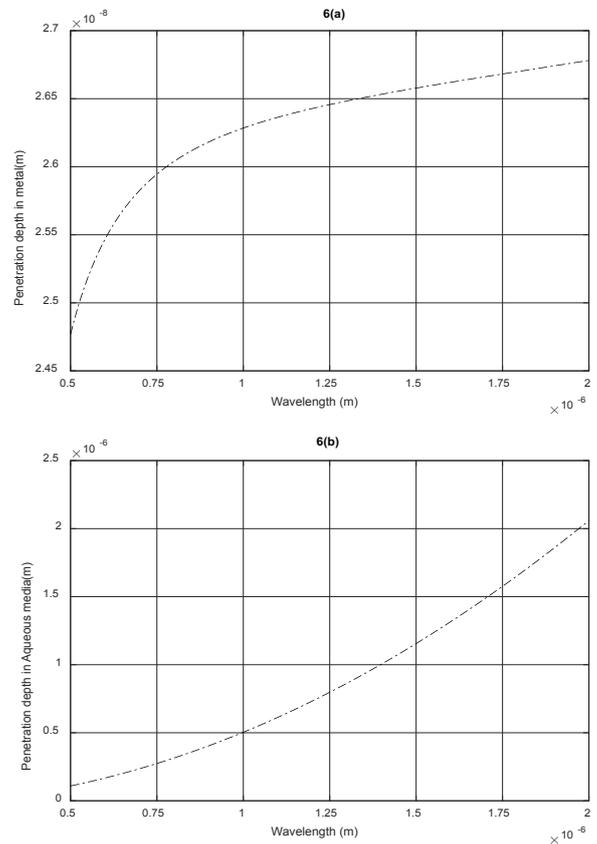
Figure 6. Penetration depth in metal (a) and aqueous media (b) at different wavelength.
