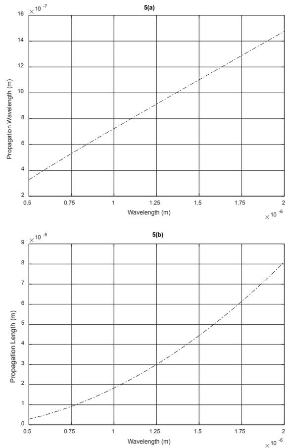
Figure 5. Propagation wavelength (a) and propagation length at different wavelength (b).
